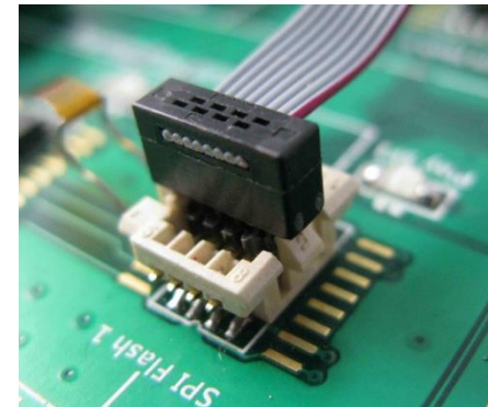
5) Plug the EM100Pro cable in the SMT connector.
